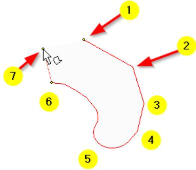
Move the mouse to new locations (2, 3 & 4) and click the left mouse button. A straight line is drawn between each click. The computer registers the exact location where you gave a click. Such a location record is called a 'vertex'. A straight line is drawn between two vertices
